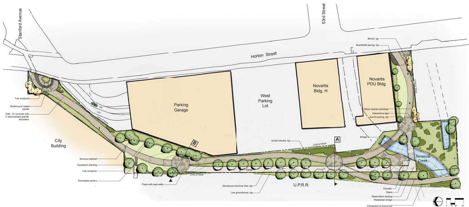
Figure 4-13 Plan for Eastern Approaches to the South Bayfront Pedestrian-Bicycle Bridge
