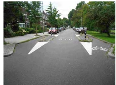
Pinchpoints allow bicyclists to avoid conflicts with motor vehicles in the narrow passageway.
