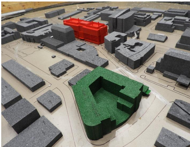
Image 2C: Wind Tunnel Study Model – Project + Cumulative Configuration
