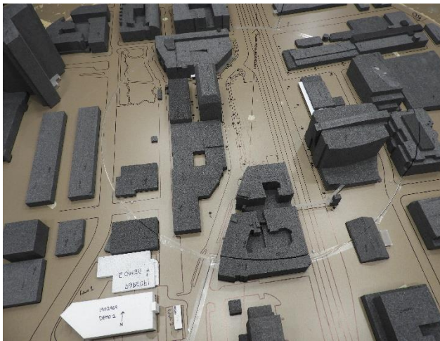
Image 2A: Wind Tunnel Study Model – Existing Configuration
