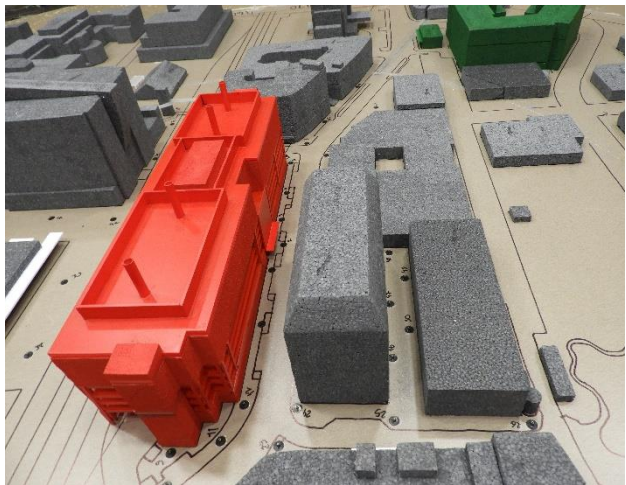
Image 2C: Wind Tunnel Study Model – Project + Cumulative Configuration
