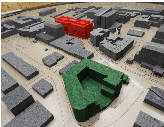
Image 2C: Wind Tunnel Study Model – Project + Cumulative Configuration
