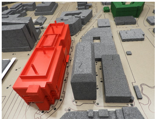
Image 2C: Wind Tunnel Study Model – Project + Cumulative Configuration
