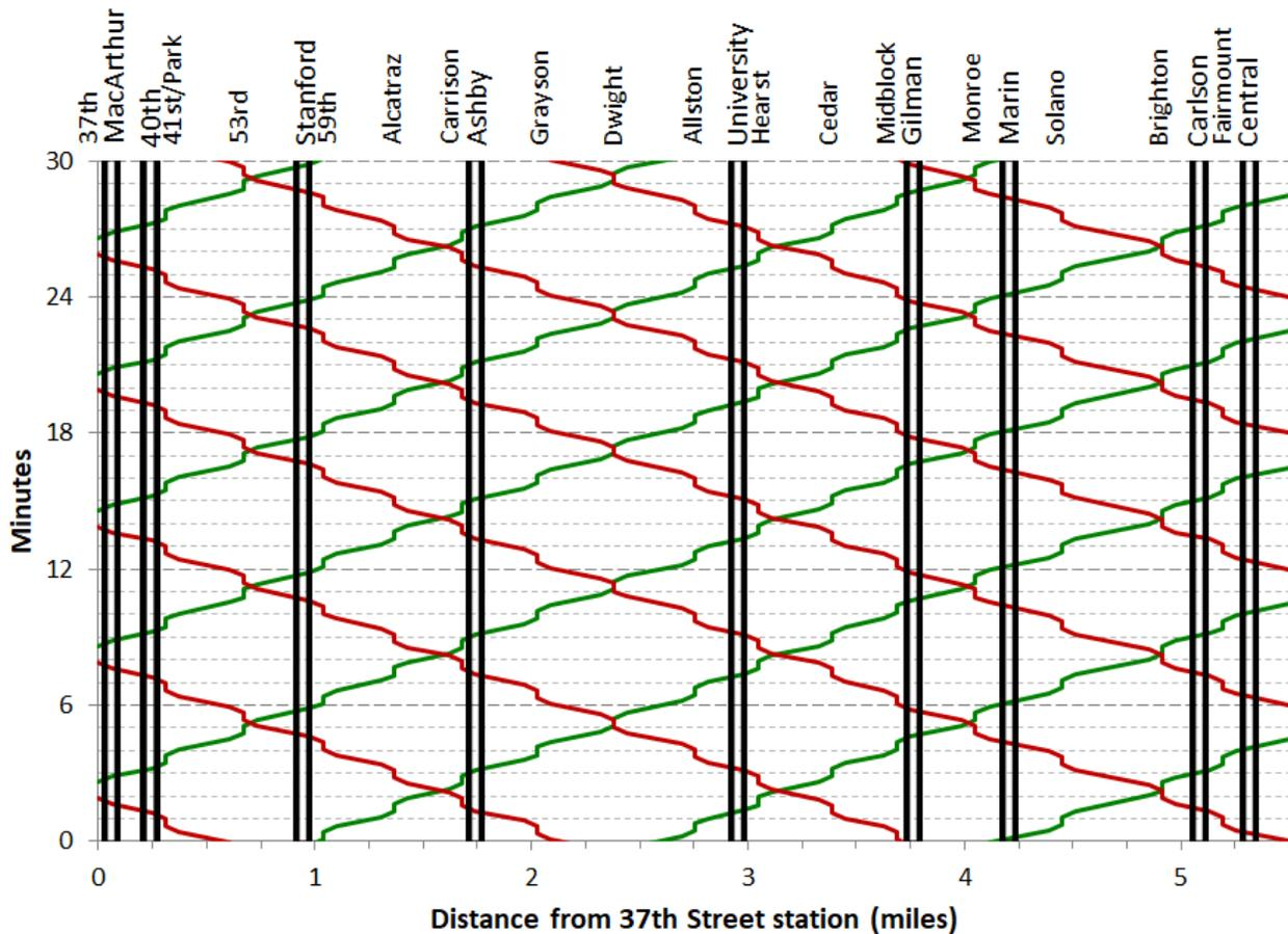
Figure 2. Time-space diagram illustrating the theoretical plausibility of single lane bi-directional bus lane at intersections with streets connecting to I-80 along San Pablo Avenue assuming 6-minute headways
