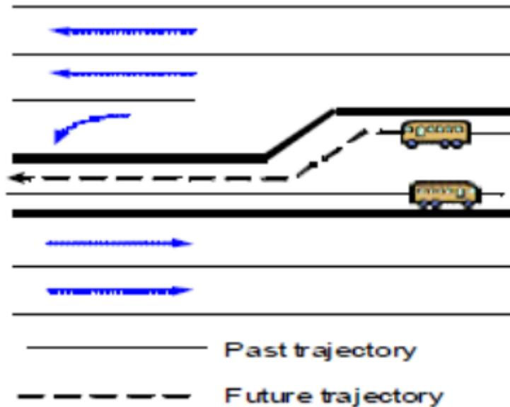
Figure 1. Schematic of a single, center-running dedicated bus rapid transit lane on one leg of San Pablo Avenue at an intersection with an arterial connected to I-80; the other leg of would also have a single dedicated bus lane (modified from <https://transweb.sjsu.edu/sites/default/files/BRT.pdf>)
